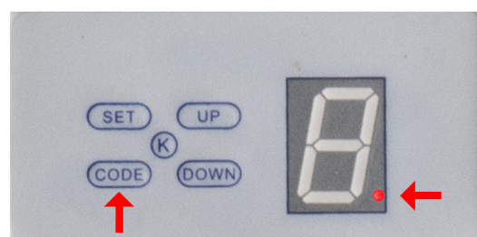
Coding LED For Programming Remotes
